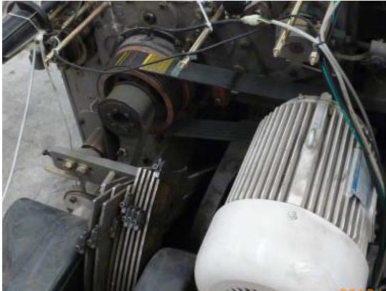
Therefore, current air jet loom requires belt replacement and drive ratio change to achieve the purpose of changing rotation speed. However, this speed changing mode brings many problems.
