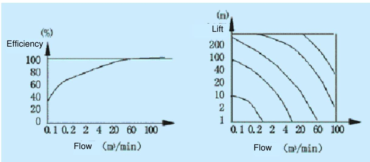
FIG. 2 Efficiency of General Standard Pump
