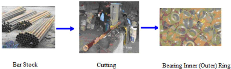
Fig. 1 Cutting of Bearing Inner and Outer Rings
