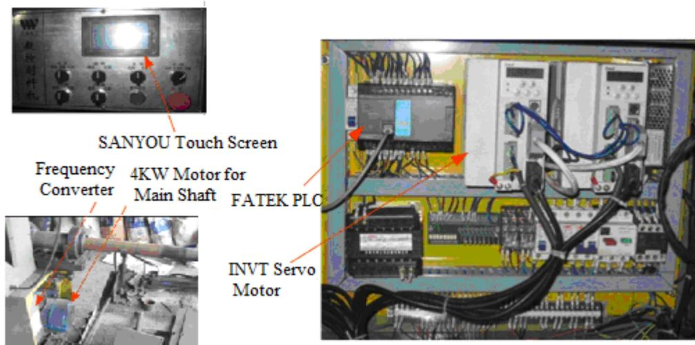
Fig. 2 Electrical System of CNC Cutter
