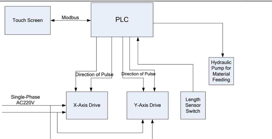
Fig. 3 Connections between Different Parts of the Electrical System
