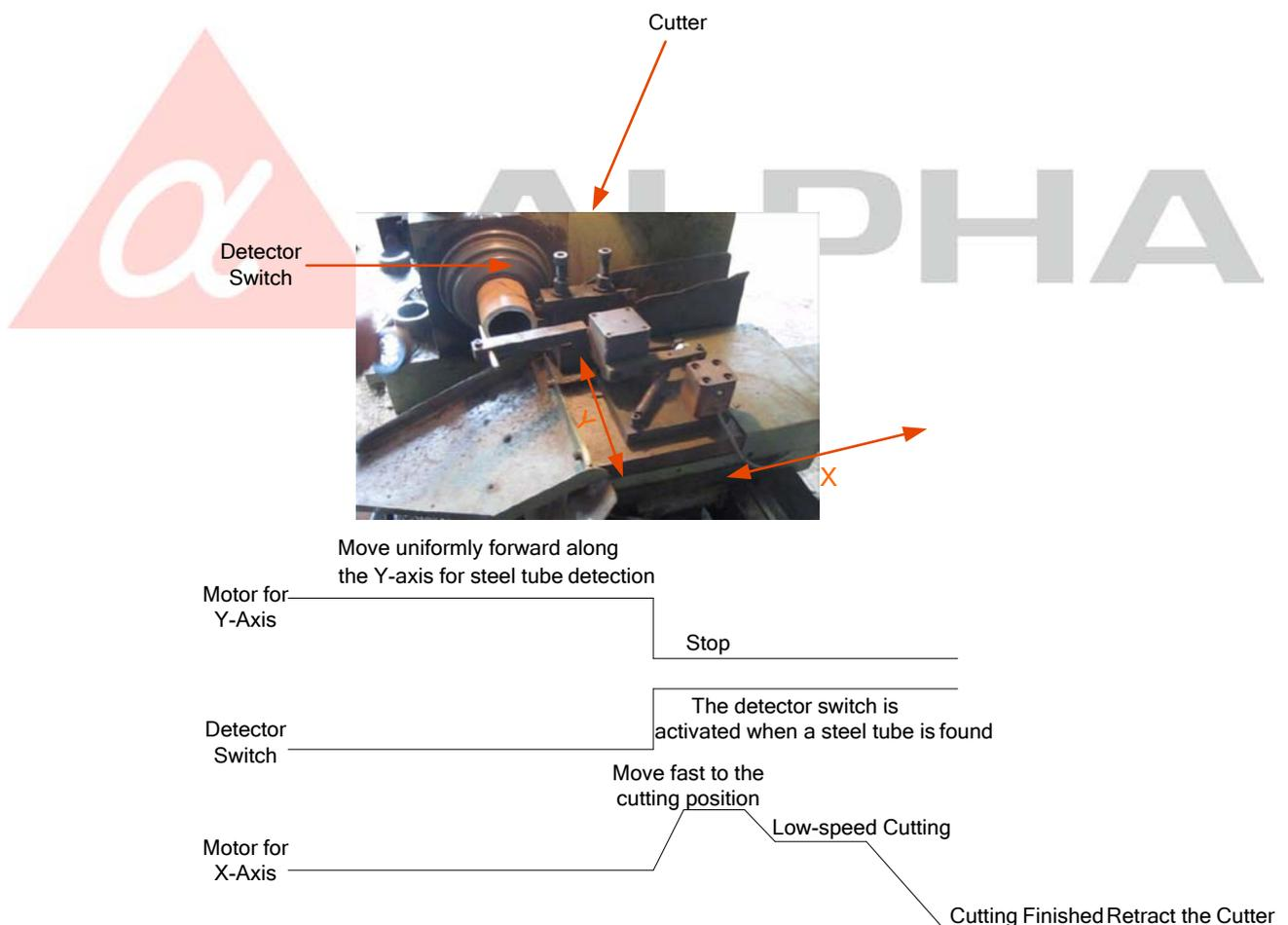
Fig.5 Process Flow Diagram
